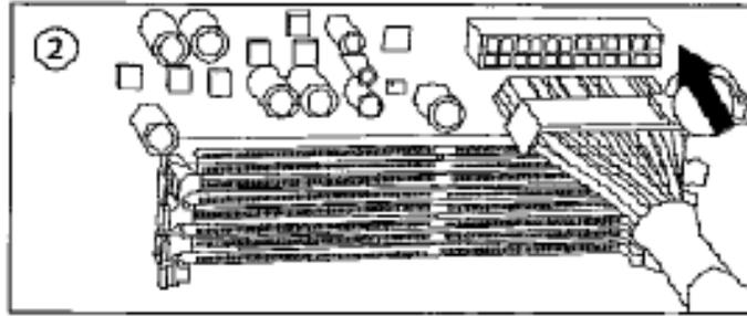
3. Connect the 8-pin or 4-pin ATX12V connector for the CPU to the appropriate connector on your motherboard. If your motherboard has an 8-pin socket with a cover on some of the openings, we recommend that you remove the cover and use the 8-pin connector.
