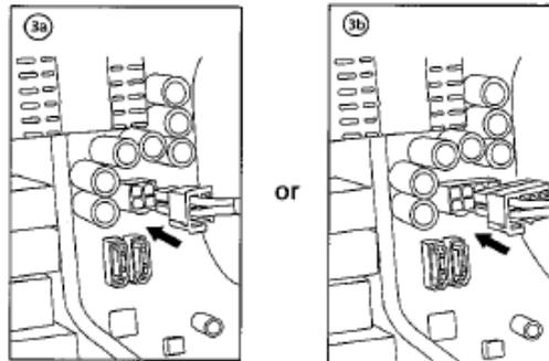
4. Connect the cables from the cable pack to the socket on the power supply as needed. If you are going to plug the additional PCI-E cable into the PSU, it should go into the red socket. If the red socket is not being used for PCI-E, then it can be used for another cable from the pack that accompanied the PSU.
